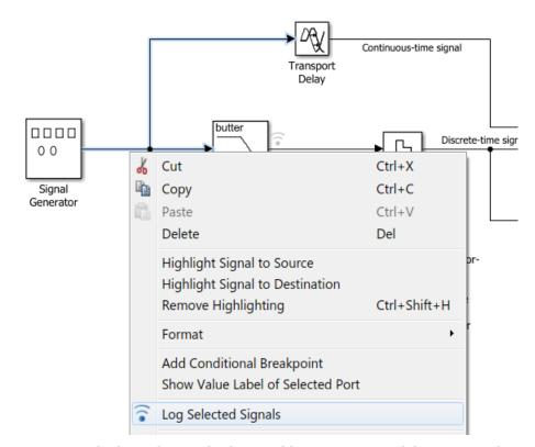
• Use any method to select multiple signal lines in your model. For example, use **Shift**+click to select multiple lines individually or **CTRL+A** to select all lines at once. Then, on the **Signal** tab, select the **Log Signals** button.
