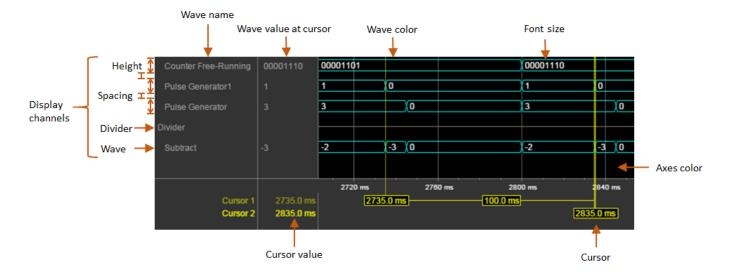
By default, when your simulation stops, the Logic Analyzer shows all the data for the simulation time on one screen. If you do not want this behavior, clear **Fit to view at Stop**. This option is disabled for long simulation times.
