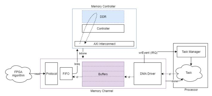
• **AXI4-Stream FIFO** – Model a connection between two FPGA algorithms through external memory. The writer puts data into the channel as a master using the MathWorks simplified AXI stream protocol and the reader receives data from the channel as a slave using the same protocol.
